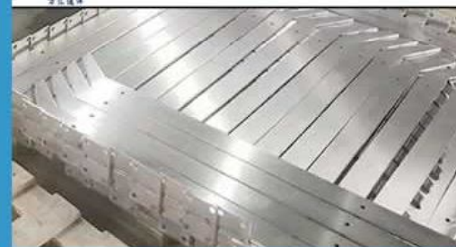
LASER CUT SS316 BALUSTRADE POST WELDING BASEPLATE
